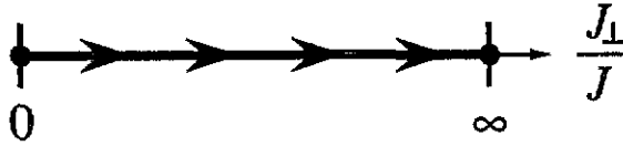
Figure 2. The conjectured renormalization-flow diagram for the Heisenberg ladders. The fixed point J_{\perp}/J = 0 is unstable with respect to the inter-chain coupling. The stable fixed point at J_{\perp}/J = \infty is described by the massive S = 0 chain for even n_l , and by the massless S = 1/2 chain for odd n_l . We thereby conclude that the whole phase of J_{\perp} > 0 is massive for even n_l and is critical for odd n_l .
